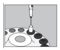
7. Slip the upper half of the **LARGE** capsule over the bottom half to completely cover the **SMALL** capsule and push down gently until locked as illustrated below:
