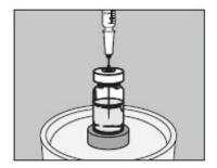
6. Inject into the center of the **SMALL** capsule through the top as illustrated below and wait for 30 seconds to allow the solution to be absorbed by the absorbing buffer:
